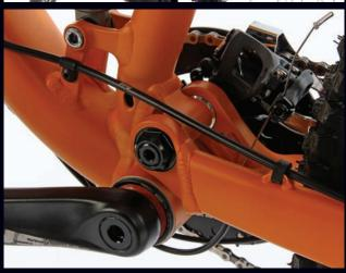
Clean, simple and tough: Kona's walking-beam, four-bar-linkage rear suspension, a direct-mount front derailleur and a coil-sprung fork.
